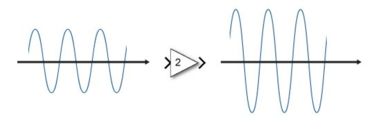
You can connect blocks to other blocks to form systems and represent more complex functionality. For example, an audio player turns a digital file into sound. A digital representation is read from storage,
